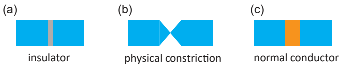
Figure 2.5. Types of Josephson junction. Different types of weak links connecting two superconductors: (a) an insulator, (b) a constriction or (c) a conductor. Adapted from Ref. [41].
