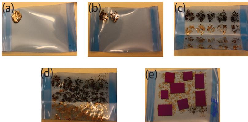
**Figure 3.2** Mechanical exfoliation process. (a) The bulk crystal with the size of around  $1\text{ cm} \times \text{cm}$  and the adhesive tape. (b) The bulk crystal was put in close contact by folding the tape and then detached from it, such that we have two footprints of the crystal (c) The footprints are duplicated by folding the tape (d) The density of flakes increased by folding the tape more times. (e) The silicon substrates put in good contact with the copy tape.
