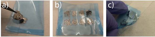
Figure 3.1. Exfoliation of 2D materials. a) Bulk crystal is tapped on adhesion tape leaving some material. b) The crystal is cleaved several times, covering the tape with random thickness flakes. c) The tape is brought in contact with a silicon wafer, depositing some flakes on its surface. Adapted from [115].
