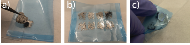
Figure 3.1. a) Bulk material is placed on the low adhesion tape and is cleaved for the first time. b) The bulk crystal is cleaved several times, which covers the tape homogeneously by thin flakes. c) The thinned down crystal is brought in contact with a silicon wafer, which leaves back crystals of various thicknesses.
