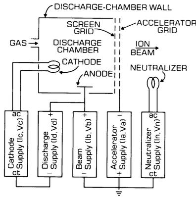
Figure 3.2: Schematics of an Ar sputtering gun.
