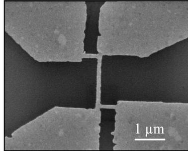
Figure 3.4: UCF gold wire (length  $1.5\ \mu\text{m}$ , width  $130\ \text{nm}$ , thickness  $20\ \text{nm}$ ).
