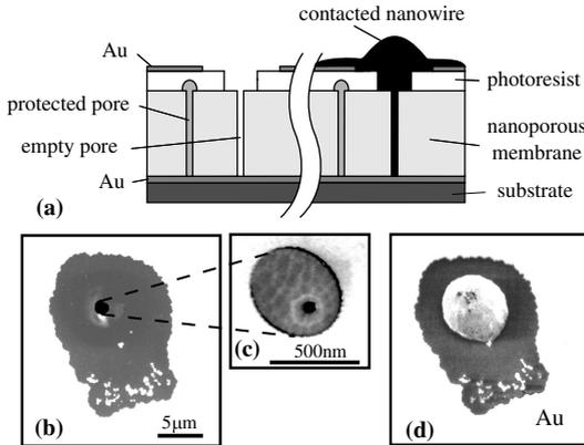
Figure A.4: (a) One selected pore with dissolved Ni protection (left) and refilled with the desired material forming an electric contact to the top Au layer (right). The SEM images are top views of one particular pore after the dissolution of Ni (b), (c) and after (partial) refilling (d).
