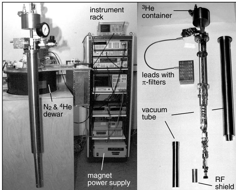
Figure 4.1: Left side:  $^3\text{He}$  cryostat with the instrument "rack". The insert, normally immersed in liquid helium, is hanging in front of the dewar. Right side: details of the insert when the tube for the isolation vacuum is removed. All the wires are connected to  $\pi$ -filters at the top of the insert.
